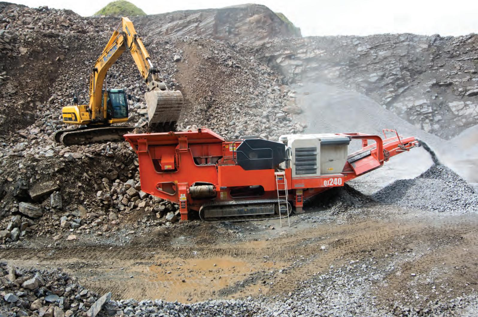
The new Sandvik QJ240 is a compact tracked jaw crusher based on the design of the world leading C-10. This compact self-propelled machine brings the revolutionary features of the Sandvik QJ340 to the smaller quarry or demolition site, where operating space is limited, yet high performance required. Of most sturdy construction, its power management coupled with unique jaw design makes it an icon for this category of crusher.
