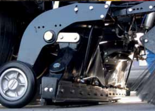
TOP High pressure deep cleaning line & gutter jet option
