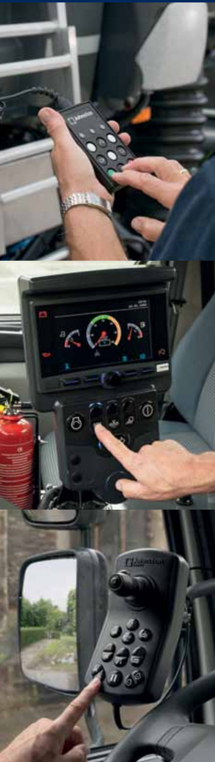
TOP Pendant control for safely raising the hopper
