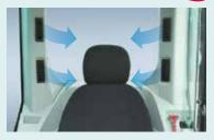
The large air-conditioner has louvers on the back pillars that blow from behind and to the right and left of the operator's seat. They can be adjusted to put a direct flow of cool/warm air on the operator, which means a more comfortable operating environment.
