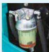
Pre fuel filter with built-in water separator
